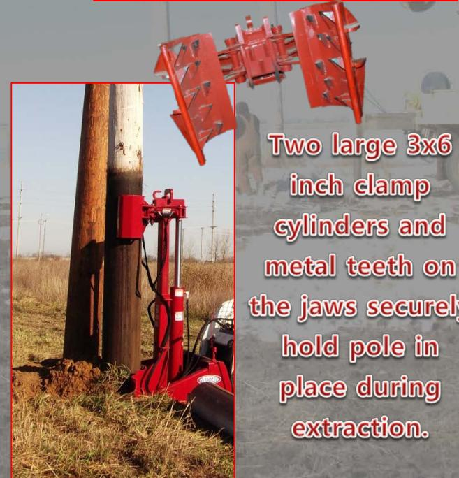
Two large 3x6 inch clamp cylinders and metal teeth on the jaws securely hold pole in place during extraction.
