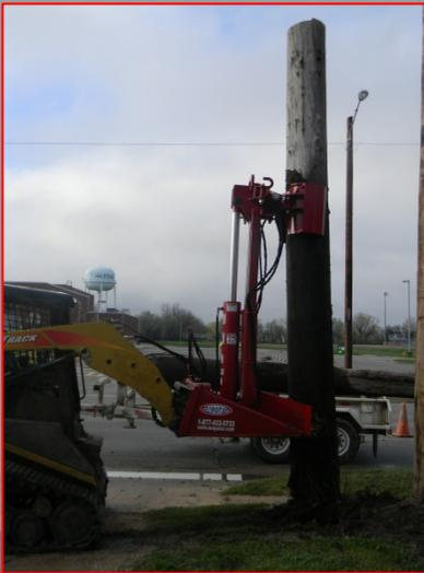
Capable of removing poles up to 90 feet in length.
